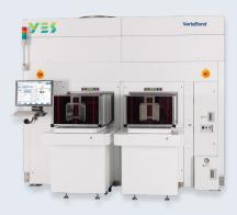
The YES VertaBond<sup>™</sup> is a production-proven automated vacuum anneal system equipped with uniform temperature control and laminar gas flow. This system has an EFEM integrated with two process modules that can accommodate 200 mm and 300 mm wafers, or panel sizes ranging from 400 mm to 550 mm. The VertaBond wafer systems can process batch sizes of 50 wafers (one PM) or 100 wafers (two PMs). VertaBond panel systems can process batch sizes of 12 panels (one PM) or 24 panels (two PMs).
